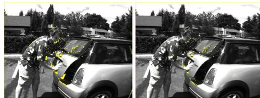
Figure 4: Left: The holes appearing in the first interpolated frame of Figure 3 after forward interpolation. Right: The remaining holes after backward interpolation.
